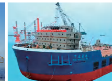
“Hengtong Lande” wind power foundation pile construction ship
